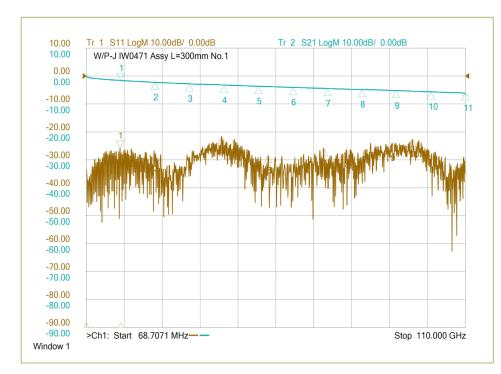
Terminated with **1.0mm** connectors designed for the 0471 cable, example test data is shown here for a 30cm/12" overall length assembly using male and female connectors:
